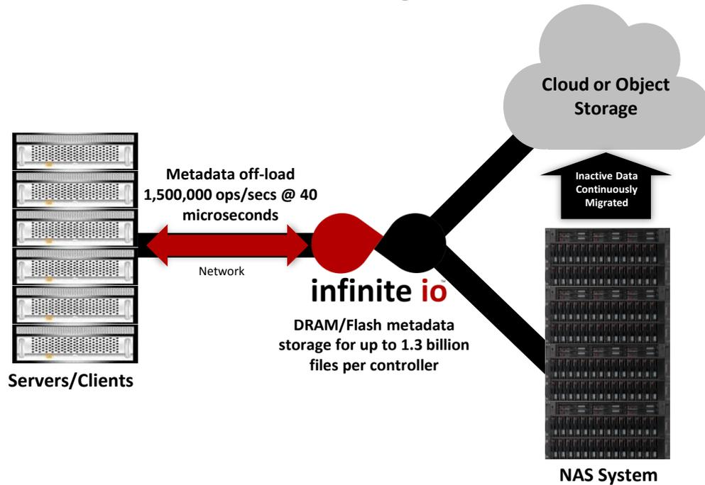
*infinite-io takes a unique approach to metadata off-load by keeping a copy of all metadata for both local and cloud migrated files in memory, making the metadata-map always “hot”*
