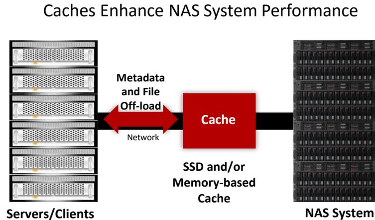
*Caches performance-enhance data and metadata that are accessed frequently. Two of the challenges of caches is the “warm-up” time, and data changing its hot/cold state.*
