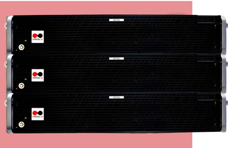
The NSC-055 is designed to sell either as a stand-alone unit or as a cluster of three accelerators with 24 10Gbps port pairs. As metadata demands increase, IT can add more appliances to the cluster. The cluster design also provides high availability, eliminating downtime or performance degradation.
